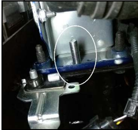
Picture B: Illustrating what the 10x40mm bolt looks like resting in place.
