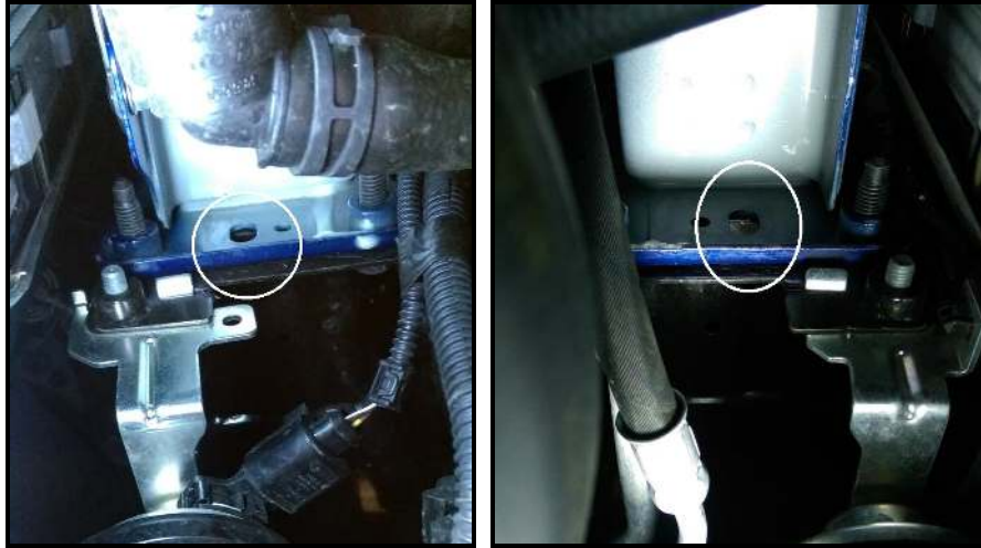
Picture A: Driver's and Passenger front upper frame hole location above both horns.
