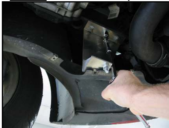
Picture G: Drivers side bracket fully installed.
